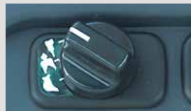
Attachment selector switch
