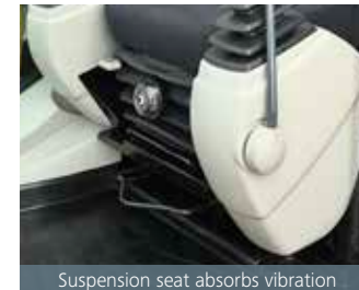
Suspension seat absorbs vibration
