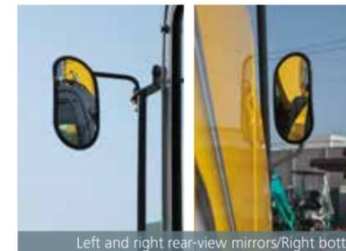
Left and right rear-view mirrors/Right bottom clearance mirror
