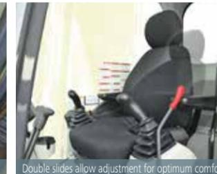
Double slides allow adjustment for optimum comfort
