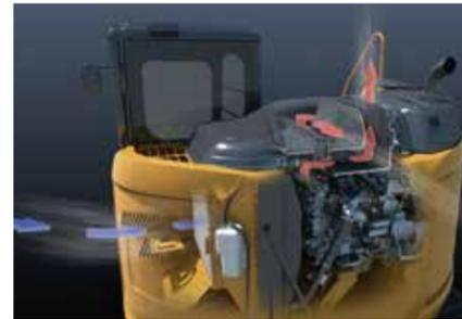
iNDr absorbs sound energy to minimize noise by making a path of air, which cools down the engine. The SK140SRD is equipped with a selective catalytic reduction (SCR) unit, which required a new design with two offset ducts on top. This allows ample space to absorb engine noise.
