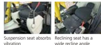
Suspension seat absorbs vibration    Reclining seat has a wide recline angle
