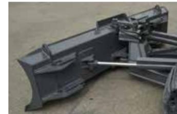
The 6-way dozer blade has Power, Angle and Tilt capability (PAT) operated from the cab. With a single control lever, the blade can be angled 25 degrees to the left or right for dispensing earth and materials away from the operator's path. The blade also tilts up on the left and right sides by 1' 6" {455 mm} for slope grading, culverts and ditches.
