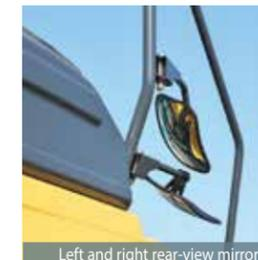
Left and right rear-view mirrors/Right bottom clearance mirror
