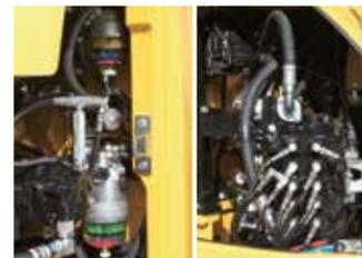
Fuel water separator/Fuel filter/Control valve
