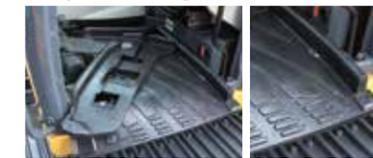
Detachable two-piece floor mat has handles for easy removal. The mat's raised edges trap dirt and grit for easy cleaning.
